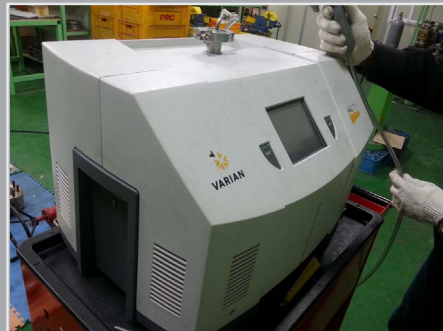
Helium leak testing – instrument sensitivity < 10^{-3} \text{ mm}^3/\text{s}
