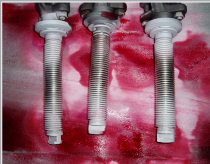
Post cycling penetrant test of bellows
