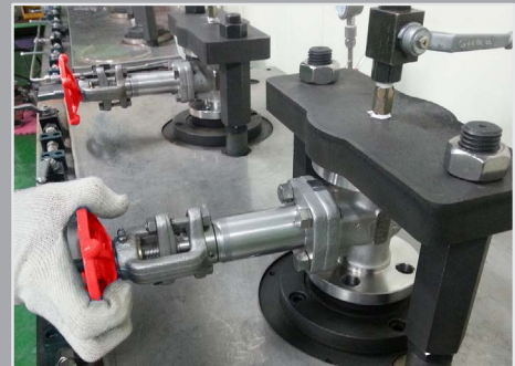
Pressure testing of each valve
